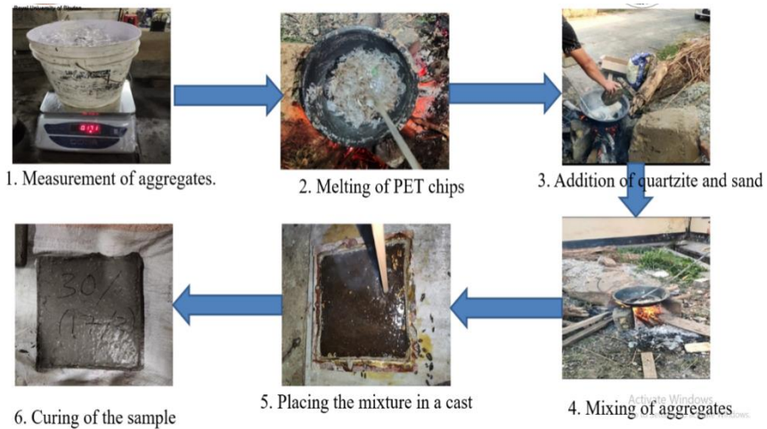
Figure 2. Production of tiles using PET binder.
